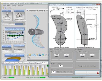
This tool allows you to create 3D models of blades with complex shapes and then export to igs 3D format... Below is a wing generating curve:
