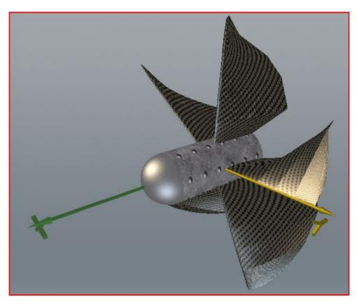
The same blade with a generator on the trailing edge (the pitching moment will be highly rearing up)
