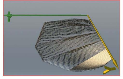
• the same blade with the generator centered at 50% of the cords profiles (pitching moment is rearing up)
